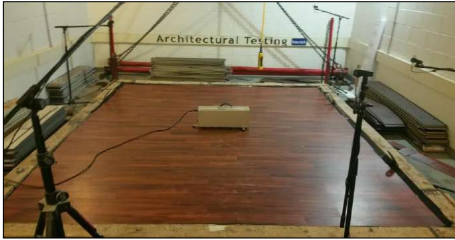
Source Room View of Test Specimen Installation
