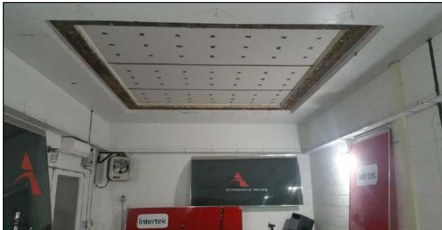
Receive Room View of Test Specimen Installation
