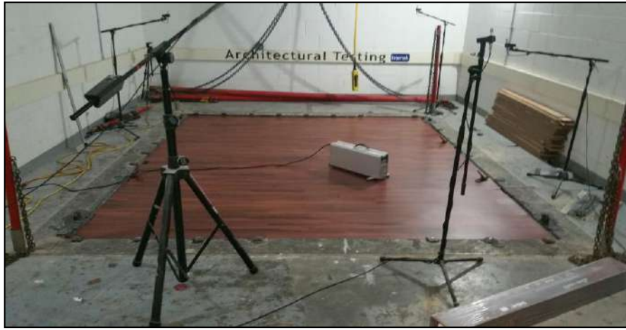
Source Room View of Test Specimen Installation
